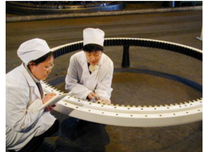
Extra-large wind energy bearing inspection
